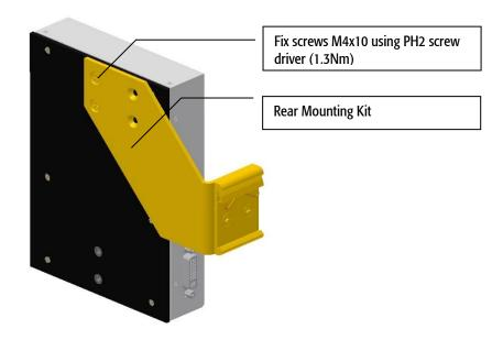
2. Mount the device to the mounting rail pushing it "down" first then "in".
