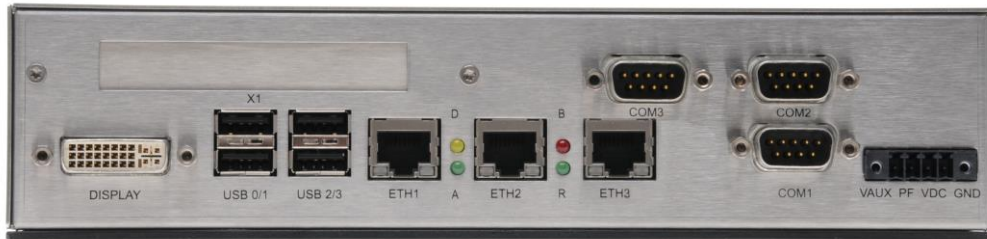
Fig. 15 Front view with connector markings (product image may vary)
