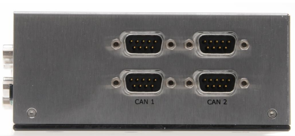
Fig. 17 Side view with connector markings (option with mounted connectivity board)
